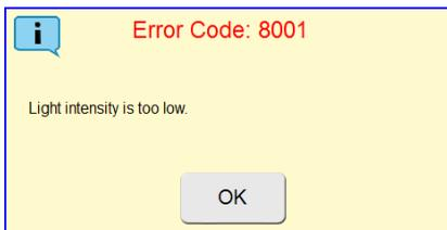
This message appears when the intensity is lower than low end limit. Try following steps to fix this problem:
